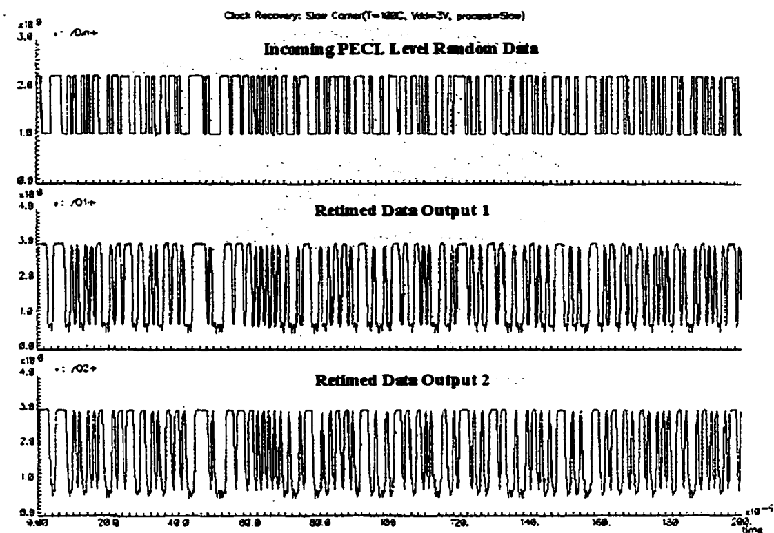
Figure 6.11 The worst case simulation results—input data and recovered data D1, D2
